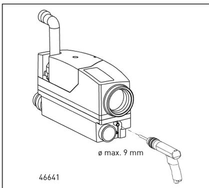
To drain the tank in an emergency, a section of garden hosepipe be connected to the tank at the bottom on the right-hand side. First, you will have to open up the 13-mm-diameter port by drilling through it with a spiral drill (maximum diameter: 9 mm). Push the hosepipe onto the port and secure it with a hose clip (tightening torque: 1.5 Nm). Make sure that the outlet opening of the hosepipe is securely sealed.
