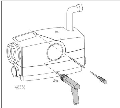
Sewage lifting units must be protected against buoyancy. The installation site should never be flooded.
