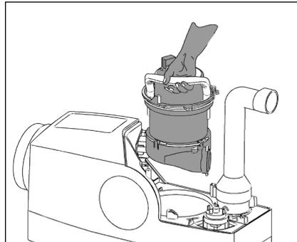
4. Remove any foreign matter from the tank and the pump through the suction opening and clean the components if necessary.
