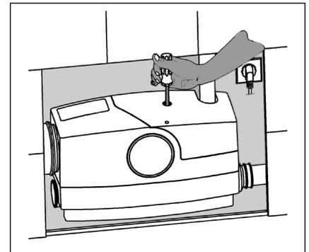
2. If the pump is sluggish or blocked, it can be set in motion again using a screwdriver, without any further disassembly. To do this, remove the stopper from the hole in the cover. Insert a long screwdriver (Torx 30 or grub-screw H5) through the hole in the cover. Turn the screwdriver gently until it engages with the slot in the motor shaft and then turn the shaft forcefully in both directions to clear the blockage.
