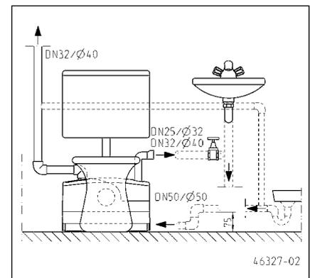
**ATTENTION!** If a connecting pipe is fitted between the WCFIX and the toilet, this will result in malfunctions. This method of installation does not comply with the approval of the Deutsches Institut für Bautechnik (the German approval body for construction products and types of construction).
