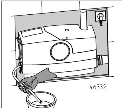
If a hose was fixed to the tank during installation, then the water in the system can be drained away quite simply through the hose and into a shallow container. The hose must then be re-sealed using a suitable stopper.
